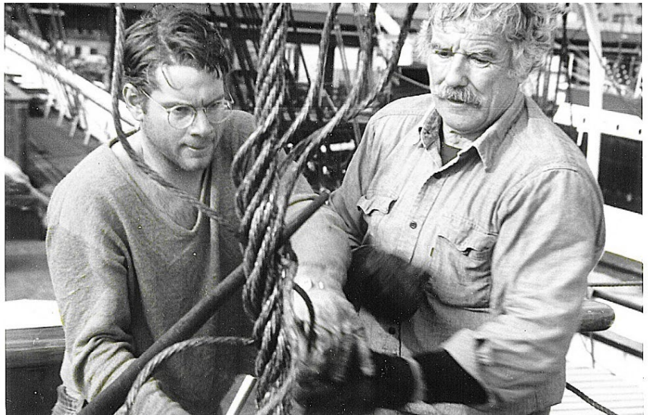
Splicing, weaving the wire into itself using a marlinspike Credit: Mr. John Atkinson
