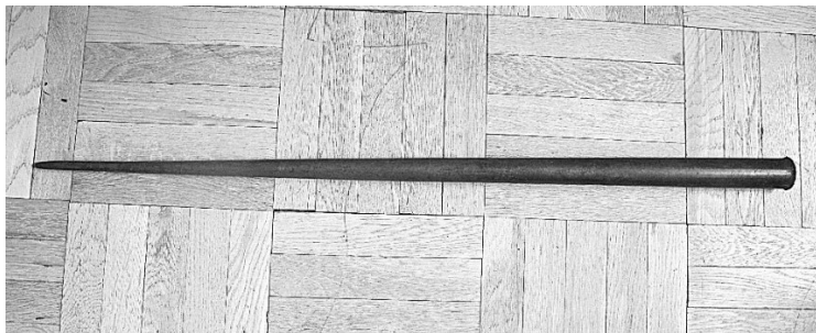
42" steel marlingspike for large wire rope Credit: Author
