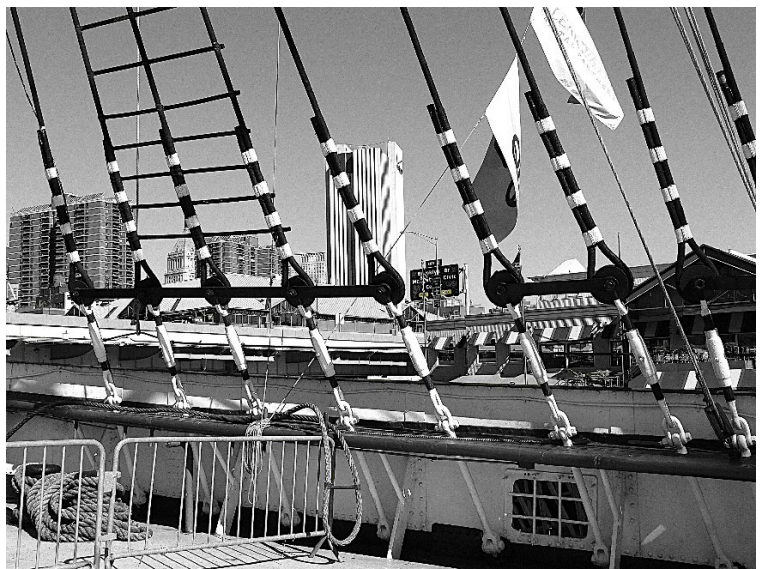
Steel standing rigging with seized ends (seizings picked out in white) Credit: Author
