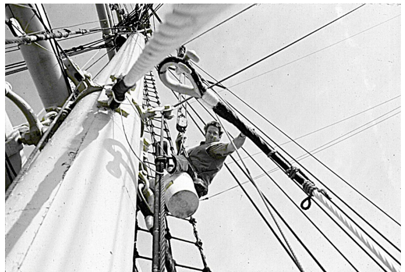
Sending aloft a spliced wire rope cap stay with throat seizing and service Credit: Author
