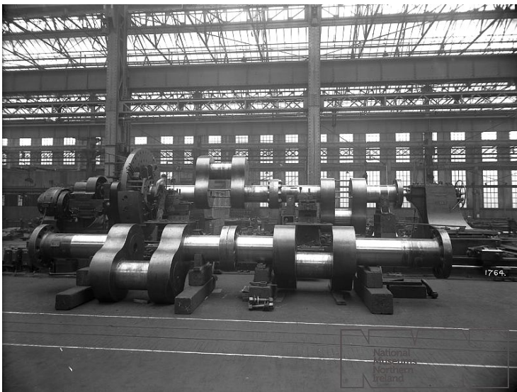
Olympic class ship crankshaft in lathe (background) Note offset crank throws Credit: Museum of Northern Ireland
