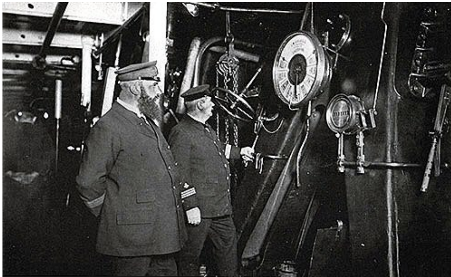
Engineers at the engine telegraph and controls on the starting platform Credit: GG Archives
